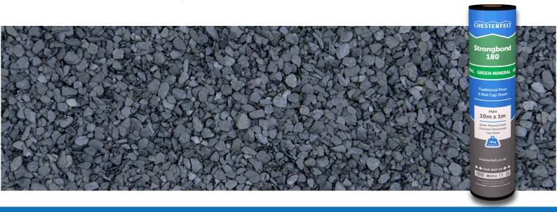
Chesterfelt Strongbond 180 Green is a traditional pour and roll cap sheet featuring a polyester core which is formed from continuous filaments and a mineral finish. Waterproofing is achieved by saturating and coating both surfaces in bitumen.
