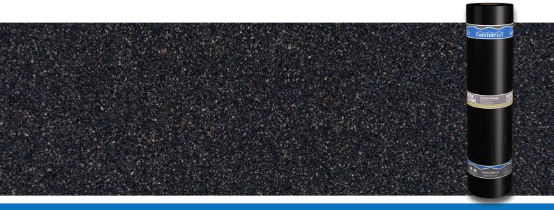
Deflector Underlay is a torch-applied underlay membrane which is designed to be used as part of a torch-applied built-up roofing system. It features a glass fibre core which is saturated and coated in bitumen and the upper surface is finished in light sand.
